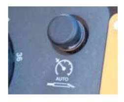
AutoDrill allows the operator to set the rotation and thrust/ pullback pressure while drilling in changing soil conditions. The patentpending Auto Resume function (pictured) allows slurry/cuttings to mix before thrust/ pullback resumes.
